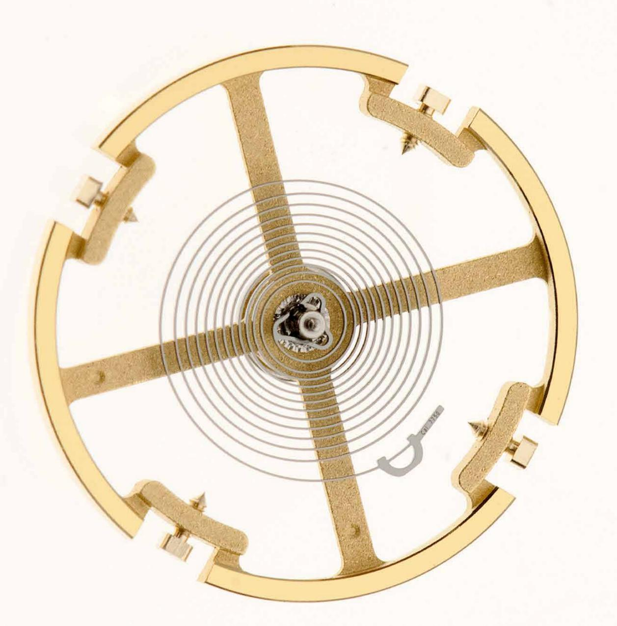
The underside of the balance wheel, the circular steel plateau with the impulse jewel pushed into it. Through this jewel, the energy is transmitted from the Swiss lever to cause the balance wheel to oscillate.
